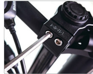
Remova os 4 parafusos
